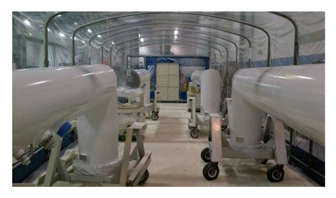
These enclosures are made from steel framing and fire-resistant PVC to contain all particulates and gases. *Photo courtesy of Duroair Technologies*.
